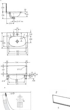
The wash basin is made of classic 18/10 stainless steel. It is supplied as standard with complete overflow arrangement and with screws and nuts for mounting on brackets. The RM 6 is not available with a factoryfitted mixer tap or drain valve. The RM 6 has folded-down rear edge.
