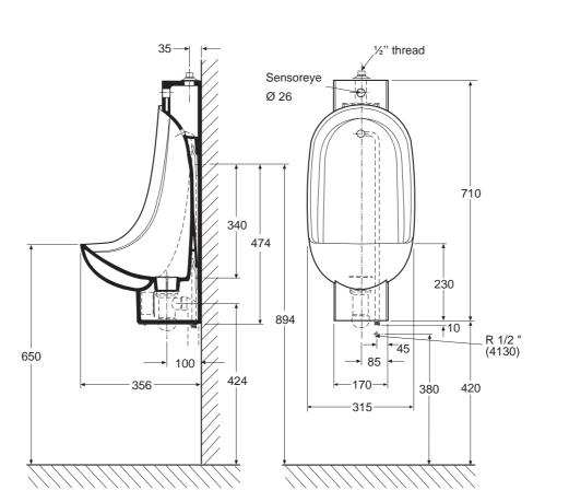
The sensor sensitivity distance is 0-50 cm. The pre-flush time is 2 seconds, with a 2-second delay. When leaving the urinal, it after-flushes for 6 seconds, with a 2-second delay. The timing and the sensitivity are not adjustable. The electronic is powered by 4 AA (6v) alkaline batteries. For more information, see the installation instruction or Ifö Sensor 100 and 150, page 6:6.
