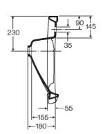
Wall outlet assembly (water trap and hose), Ifö no. 98050 for 2642-0031 and 2642-1731.
