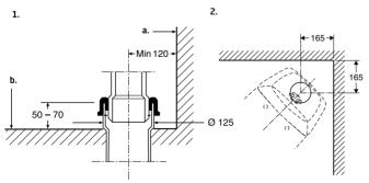
1. Mounting perpendicular to floor. a. Ready wall b. Ready floor 2. Corner installation
